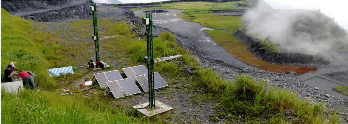
Figure 4. TAROGE-II tower structure. TAROGE-II includes three towers structure and each tower carry two dual-polarized LPDA antennas with a 2.5 meters spacing. This figure shows two towers and a 800W PV array system are placed in between of them.
