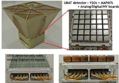
Fig. 3. The assembled UBAT and its detector.
