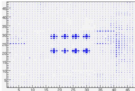
Fig. 4. The response of the UBAT detector to the collimated Am-241 X-ray source.
