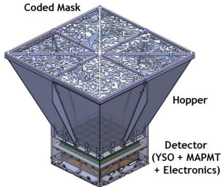
**Fig. 1.** The UFFO Burst Alert & Trigger Telescope.
